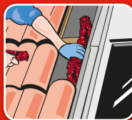
Adhering tiles to roof windows
