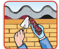
Sealing of corrugated roofs
