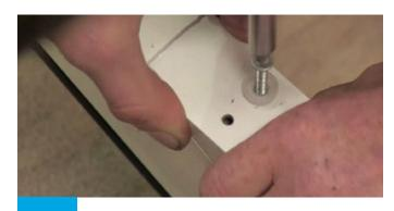
Fix the gusset with screws provided and cover with screw caps.
