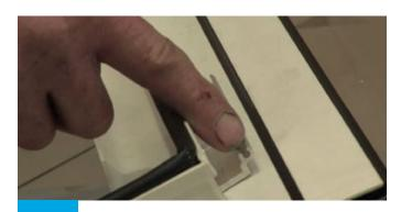
The hinge channel fits over the outer frame hinge.
