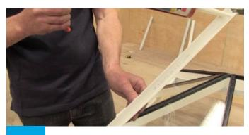
Seal both sides of the internal female muntin bar close to the internal edge. Always use the correct sealant.
